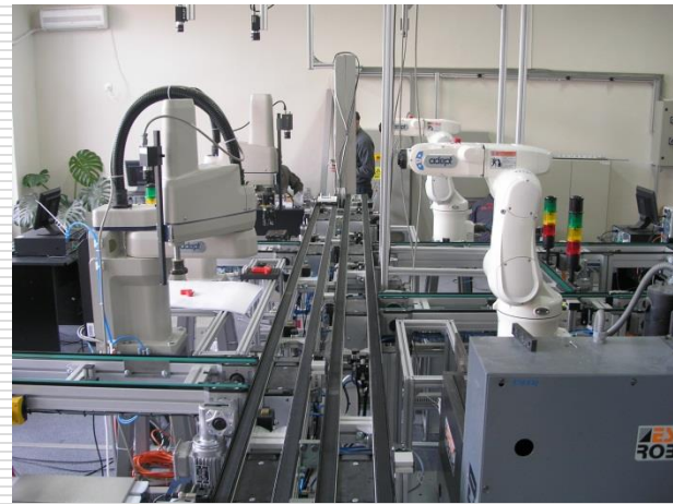
Layout of the manufacturing cell with holonic control (Shop floor robot-vision manufacturing platform at CIMR)
