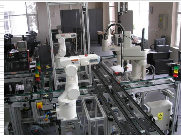
Layout of the manufacturing cell with holonic control (Shop floor robot-vision manufacturing platform at CIMR)
